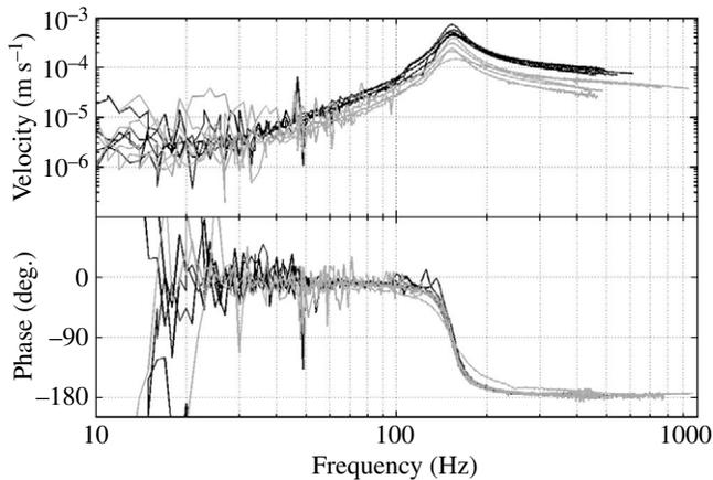
Fig. 8. Relative ossicular response at the distal tip on the malleus head in line with the stimulation direction of the same five right ears for lateral (black) and vertical (gray) stimulation. Each frequency response was shifted along the logarithmic frequency scale to bring the resonant frequencies into alignment at an arbitrary frequency of 150 Hz. Over the frequency band tested, malleus velocity amplitudes in response to lateral stimulation exceeded those in response to vertical stimulation.
