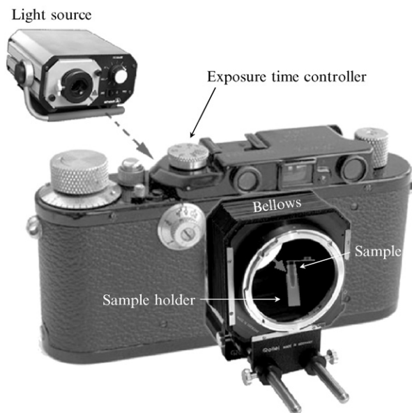
FIG. 3. Schematic cross-linking system. The reaction mixture is prepared in a polymerase chain reaction (PCR) tube (see Note 3) immediately before irradiation. A glass vial is used to hold the PCR tube within the dark chamber (bellows). The sample is illuminated through the open back of a camera body using the camera shutter mechanism to control the illumination time.
